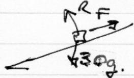
$$\begin{aligned} & \text{loss of PE} \\ & = 1500g(\sin 20^\circ - \frac{1}{4}g \cos 20^\circ) \\ & = 1574J \\ & = \frac{1}{2}mu^2, \therefore u = 10.24 \text{ m/s} \end{aligned}$$
