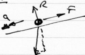
$$\begin{aligned} F &= \frac{30}{4}g \cos 20^\circ \text{ as before} \\ \text{Resolve } \leftarrow & 30g \sin 20^\circ - F = ma = 30a \\ \therefore a &= g \sin 20^\circ - \frac{1}{4}g \cos 20^\circ \end{aligned}$$
