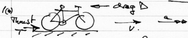
$$\text{Power} = \text{force} \times \text{speed}$$
