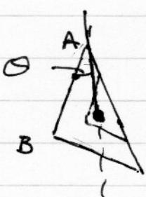
$$\begin{aligned} & 36 - 11 = 25 \\ & \tan \theta = \frac{11}{25} \quad \therefore \theta = 23.75^\circ \\ & \approx 24^\circ \end{aligned}$$
